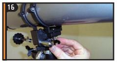
Reattach both wingnuts and tighten to secure in place.
