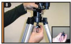
From underneath the tripod mounting platform, thread the mounting bolt with washer into the threaded hole on the bottom of the equatorial mount.
