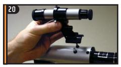
Orient the finderscope so that the large lens is facing towards the front of the tube. Place finderscope over the posts on the tube and tighten it down with the knurled nuts.
