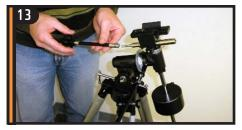
The longer cable should attach to the Right Ascension axis and the shorter cable attaches to the Declination axis as shown above.
