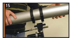
Place the tube on the mount by lining up the screws with the mouting holes on the mount. The dec cable should be extending towards the focuser end of the telescope tube.
