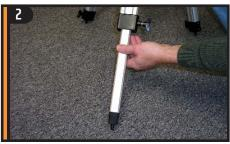
To set up the tripod, spread the legs outward until they are fully extended. Extend the center portion of each of the three tripod legs down 6-
