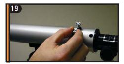
Locate the finderscope. Remove the knurled nuts on the threaded posts at the focuser end of the telescope tube.
