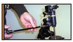
Slide the chrome end of the slow motion control cables onto equatorial mount gear shaft and tighten set screw to secure in place.
