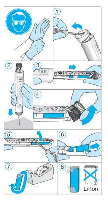
Open the handle as shown, remove the battery and dispose of it according to local environmental regulations.
