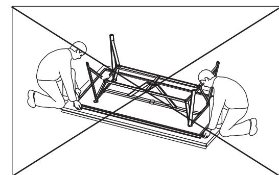
Do not use any table leg as pivot point to turn over the table.
