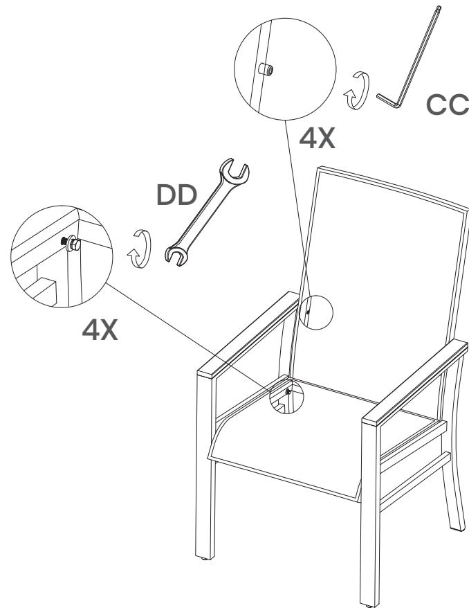
Note: After positioning the product correctly, ensure that all four legs are level with the ground, and then use a wrench to tighten the bolts.
