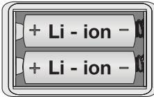
Batteries are located in the battery housing behind the light fixture. Select the OFF position on the light prior to opening the battery housing. Remove the four screws to reveal the batteries.
