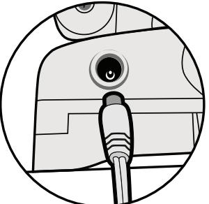
Connect the wire from the solar panel into the socket located under the light fixture. Your solar motion light will now begin to charge.
