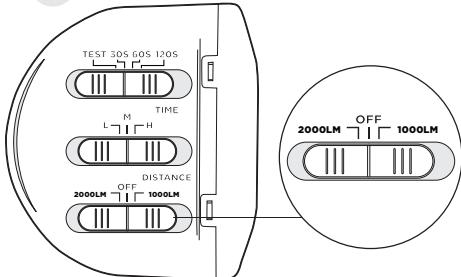
Prior to using your solar motion light, the solar panel needs to be connected to the light for a period of three days. This initial charge should be done in the OFF position. After the third day, your included batteries will be fully charged and your solar motion light is ready for operation.
