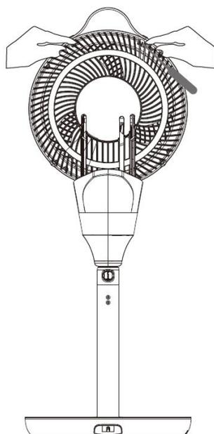
2. Squeeze the two tabs to the left and right of the screws and pull away. At the front of the fan blades there is a locking cap – unscrew the cap in a clockwise motion to remove the fan blades.
