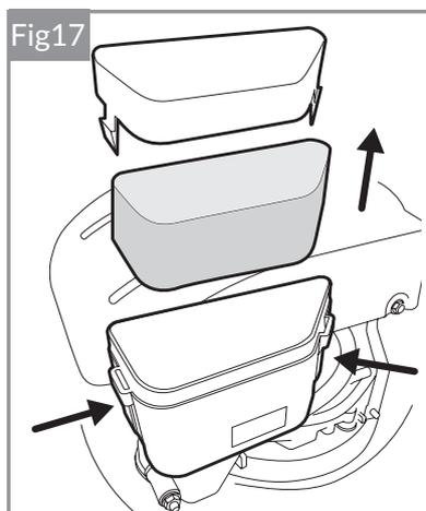
**WARNING!** Do not twist the foam cartridge to clean it as this could cause damage. If your mower is not serviced correctly, you could reduce your mower's ability to operate and void warranty.
