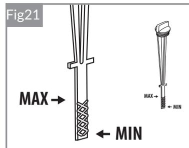
in. Remove the dipstick and check the oil level holding the dipstick horizontal.
