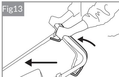
forward move the Drive Lever up and forward (Fig. 13). The mower can be pushed with the drive disengaged for more precise handling. After mowing and emptying the Grass Collection Bag ensure the engine is not running and turned off.
