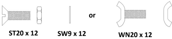
Rear View (attach nuts and bolts or wing nuts from rear)
